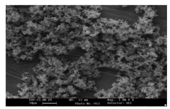
Figure1: Electron-microscopic images of molecularly imprinted polymer particles-magnification 1.00 KX, with particle diameter 10 μm.
